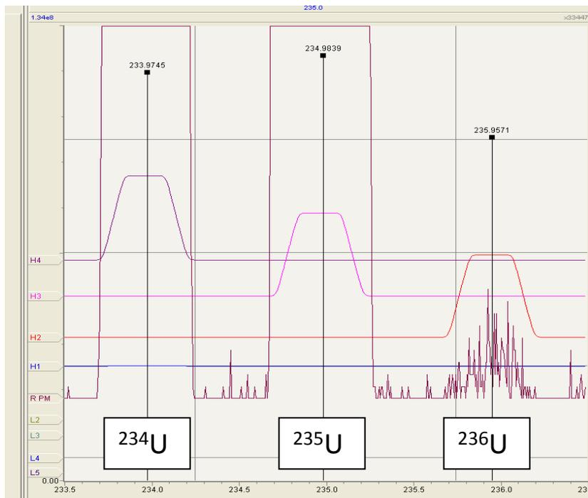
Figure 1. Mass scan showing Faraday/Daly coincidence.
