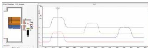
Mass scan of SRMU500 showing unit mass separation with respect to uranium.
