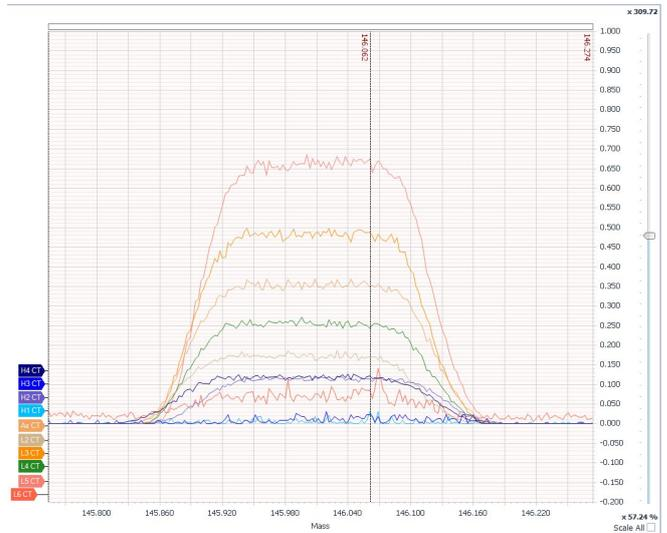
Figure 2. Ion counter shapes at Nd spacing.
