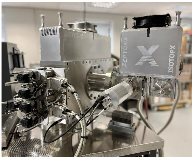
Figure 1. Phoenix TIMS collector equipped with (from left to right) an array of 9 ATONA® Faradays, WARP filter, ion counting Daly and Zeptona rear Faraday.
