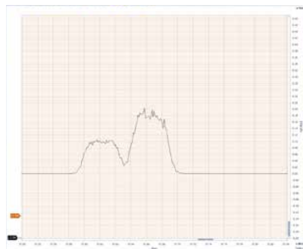
Fig 6. shows the complete peak separation of ^{40}\text{Ar} peak from the \text{C}_3\text{H}_4 organic peak
