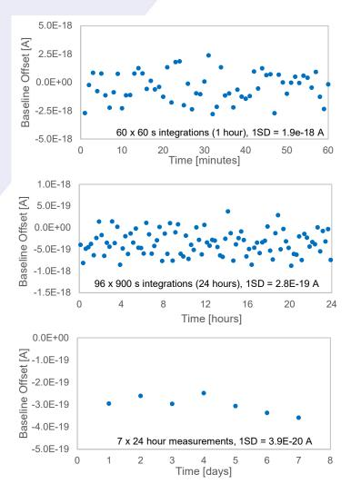
Figure 3. Zeptona baseline offset over 1 hour (top), 24 hours (middle) and 7 days (bottom).
