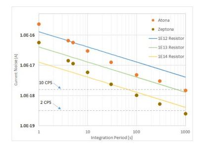
Figure 2. Noise characteristic of the Zeptona and ATONA® amplifiers, with resistor amplifier performance for reference.
