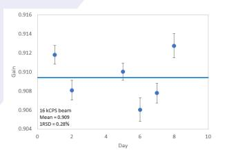
Figure 6. Ion counter stability relative to a Faraday over 8 days.
