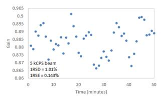
Figure 8. Gain calibration profile of an ion counter relative to a Zeptona Faraday with a 5 kCPS beam
