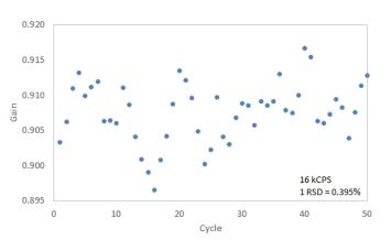
Figure 5. Ion counting stability relative to Zeptona Faraday over 60 minutes
