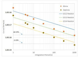
Figure 7. Noise characteristic of the ATONA® and Zeptona amplifiers.
