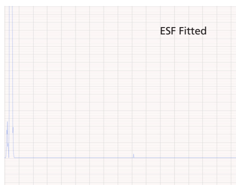
The scans above show the differences in the baselines over the mass range 3amu to 3.5amu, without and then with an ESF. The peaks on the far left are ^3\text{He}^+ and \text{HD}^+/\text{H}_3^+
