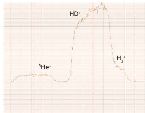
The resolution of the NGX Helium Plus allows comfortable separation of the ^3\text{He}^+ from the \text{HD}^+/\text{H}_3^+ interferences
