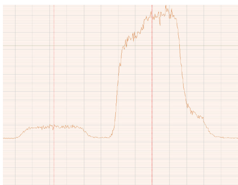
Fig 4. The ^3\text{He} peak is clearly mass resolved from the HD molecule. This is only possible due to the inherent large mass resolution of the NGX. This scan on the multiplier shows the ^3\text{He} (on the left) fully mass resolved from the HD molecular peak on the right. There is no evidence of the ^4\text{He} peak tail which would be apparent on the right of the scan. Note the width and flatness of the ^3\text{He} peak, this makes it ideal for accurate ^3\text{He} determination.
