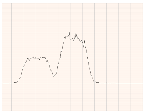
Fig 6. shows the complete peak separation of ^{40}\text{Ar} peak from the \text{C}_3\text{H}_4 organic peak
