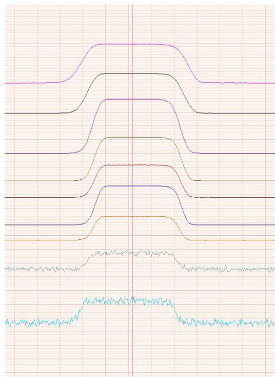
Fig 1. The figure shows coincidence of all nine isotopes of xenon. The ion optics of the NGX permits the simultaneous measurement of all the xenon isotopes.
